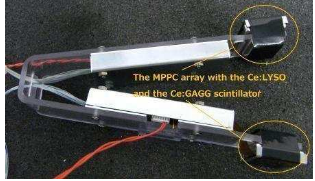
Fig. 6. Photo of the developed tweezers type coincidence imager using a pair of MPPC arrays coupled with the 0.5 \times 0.5 mm 2 Ce:LYSO and Ce:GAGG scintillator matrices.
