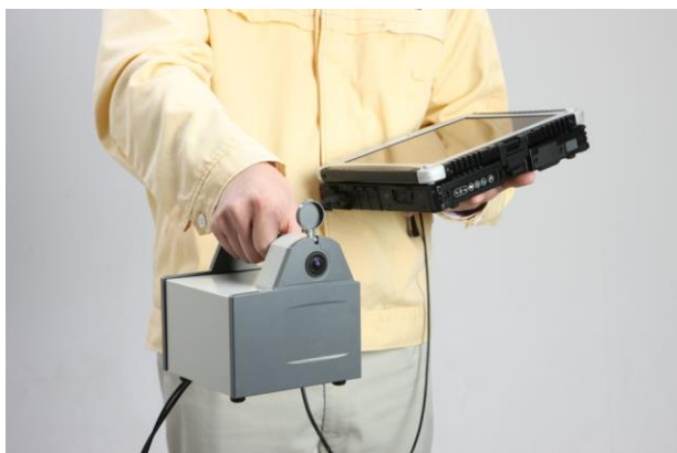
Fig.14 Photo of the handy Compton camera prototype currently being fabricated by Hamamatsu Photonics K. K. Its weight is only 1.9 kg!
